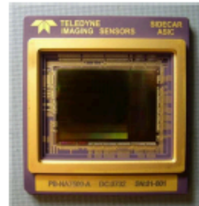
Hubble Space Telescope SIDECAR ASIC package (Hermetically Sealed)
