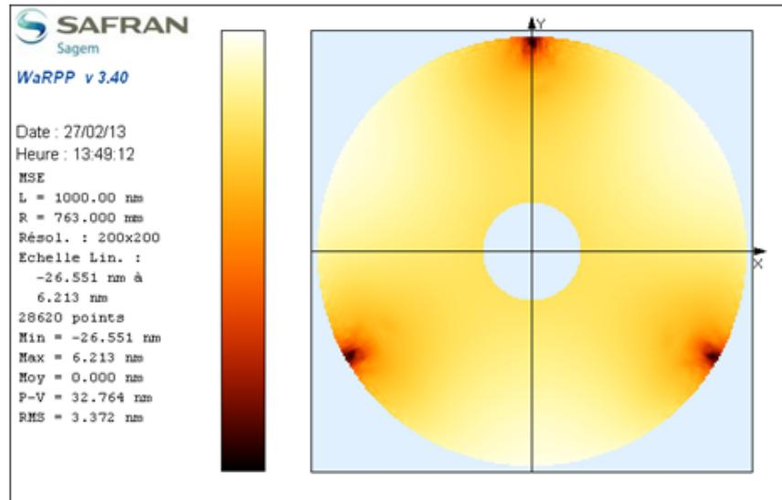
Difference RMS 6.6nm in wave-front error
