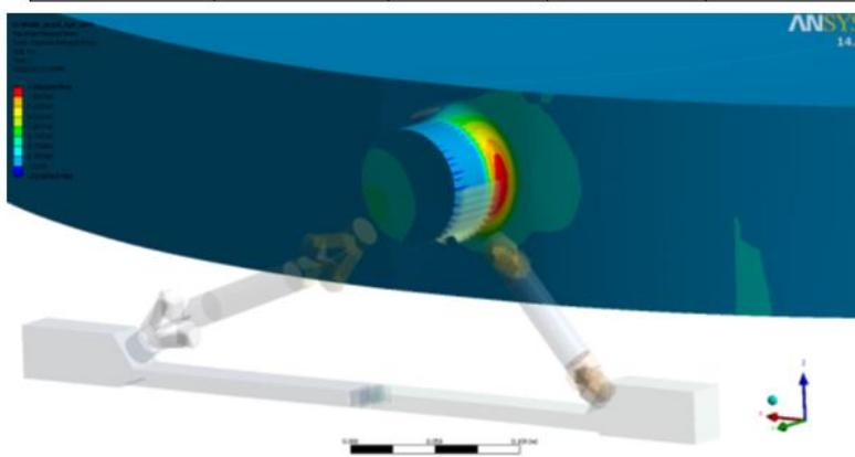
Stress in glass @ RT + launch inertial loads
